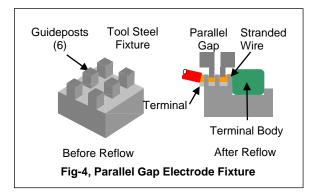
Place the terminal body on the Tool Steel Fixture. The terminal leads should cover and touch the bottom electrode or fixture surface with minimum contact force. Next, place the stranded wire over each terminal. The guideposts captivate the stranded wire. Complete the reflow by contacting the stranded wire with a flat rectangular electrode.
