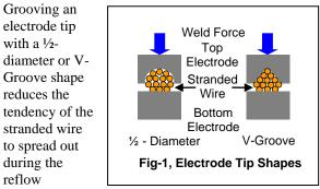
soldering process. Fig-1 shows an opposed electrode configuration, but this process also works with the parallel gap electrode configuration. IMPORTANT - Shaped electrodes will NOT prevent all wire strands from separating from the main wire bundle.
