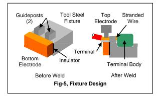
Place the terminal body on the Tool Steel Fixture. The terminal leads should cover and touch the bottom electrode surface with minimum contact force.
