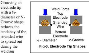
process. See Fig-3. IMPORTANT - Shaped electrodes will NOT prevent all wire strands from separating from the main wire bundle.
