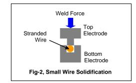
The final solidified wire mass can then be resistance welded to a terminal using a rectangular or round, flat tip electrode. The flat tip is easy to clean, which is a major advantage of this method. Two welding systems are required, one to solidify the wire and a second system to weld the solidified wire to the terminal. The two welding systems represent a minor disadvantage.
