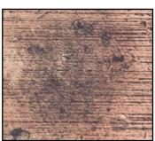
The last photo shows both nickel build-up and copper pitting on the electrode tip face after 100 welds.
