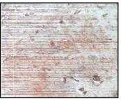
This photo shows same electrode tip surface after making 30 welds on two 0.12 mm thick Nickel Alloy 200 parts.
