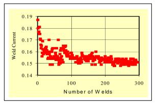
After many welds, the electrode tip surface eventually becomes so heavily pitted, oxidized, and covered with part plating and part material that the heat generated in the weld is adversely affected, resulting in degraded weld strength.
