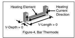
Both thermode configurations can be pulsed or constant temperature heated. A Type K thermocouple welded to a location closest to the contact face provides temperature feedback and some resistance to chemical attack by flux fumes.
